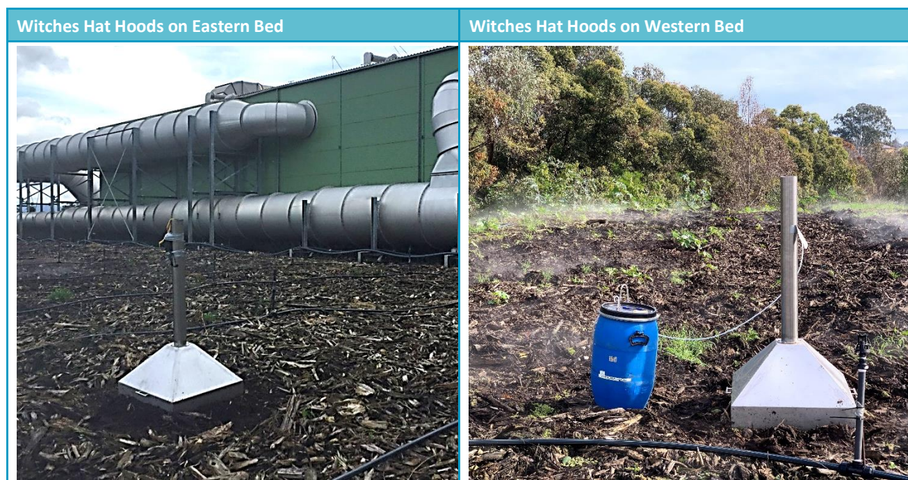
Figure 1 Illustration of Witches Hat Hoods being used on EFS Biofilter Beds
